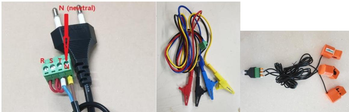
If you want to measure single phase with 3-channel display by using 3 current clamp, please make the cable connection as the above photo left.
